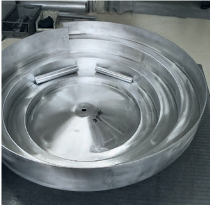
— Conventionally-made bowl feeder – welded, bent, and ground in stainless steel
