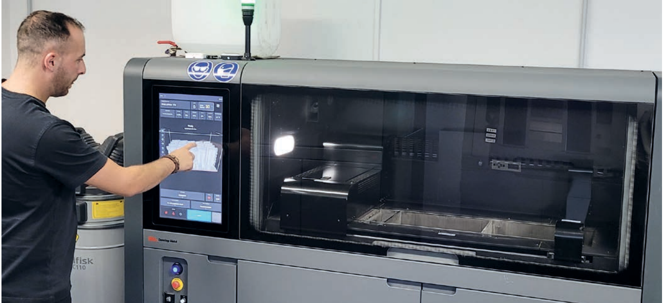
— The production of feeding and assembly components at IFC using the Desktop Metal Shop System™, the high-speed and high-resolution binder jetting system
